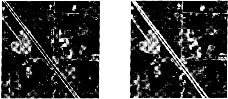
Figure 2-11 The DILATE function has been used to fuse the visual elements of this 512-by-512 aerial image.
